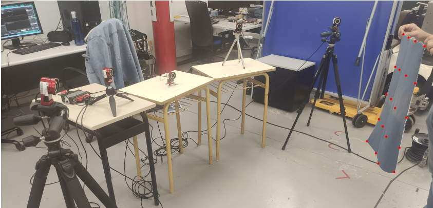
Figure 4.12: Setup used to record the motion of the textiles: 5 cameras surround the scene so that every marker (highlighted in red in the photo) is visible to at least 2 cameras at the same time. This ensures that the system can be certain of the 3D position of the marker.
