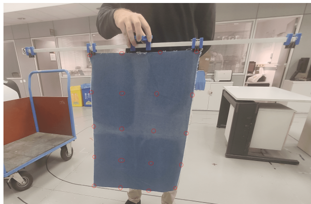
Figure 4.11: Reflective markers attached to the denim sample (encircled in red). The markers are very small, with a diameter of 3 mm and a weight of 0.013 g. We use 20 reflective markers when the size of the textile is A2 and 12 when it is A3.
