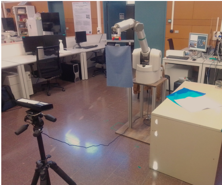
Figure 4.2: Experimental setup for the recording of the motion of the real textiles. On the left, the depth camera. On the right, the robotic arm with an affixed hanger.
