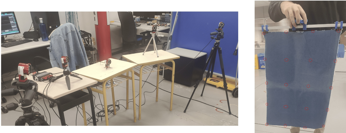
Figure 2. Left: setup used to record the motion of the textiles. Five cameras surround the scene so that every marker (encircled in red on the right) is visible to at least 2 cameras at the same time. Right: reflective markers attached to the denim sample, with a diameter of 3 mm and a weight of 0.013 g.
