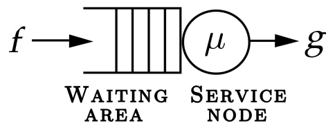
Figure 3.1: Example of a system with a queue and a server of speed \mu .
