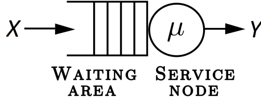
Figure 1: Example of a system with a queue and a server of speed \mu .
